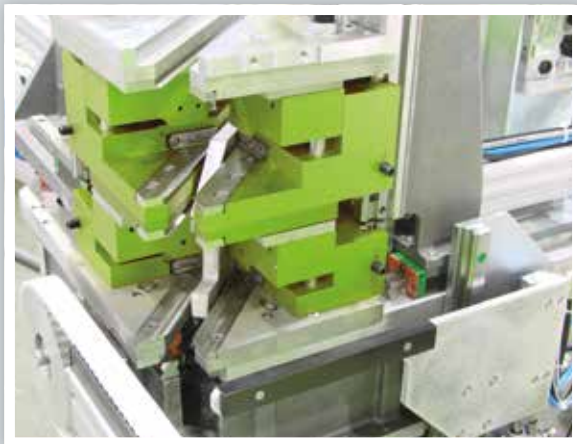
Duplex-Schweißen duplex welding
